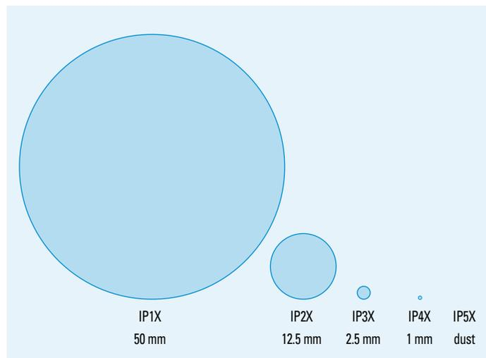
To get some notion of how big the "foreign objects" being described in each of these ratings really are, the diagram above illustrates actual particle sizes. It shows that an AED like the Philips HeartStart OnSite, because it has a rating of IP21, is in danger of being compromised by a small pebble about 12.5 millimeters (mm) in diameter.
