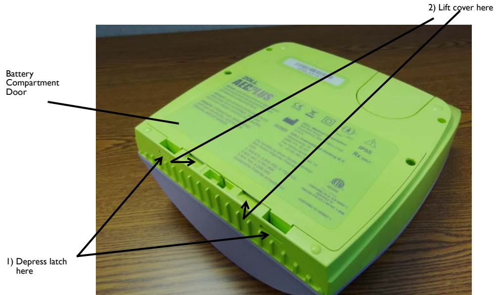
Figure 7: Removing the Battery Compartment Door
